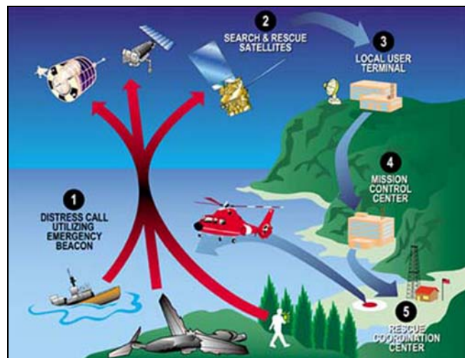
Figure 6a. COSPAS-SARSAT System Overview (NOAA Satellite and Information Service, 2005).
